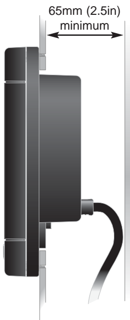
Fig 4.2 - Clearance Required Behind Bulkhead
