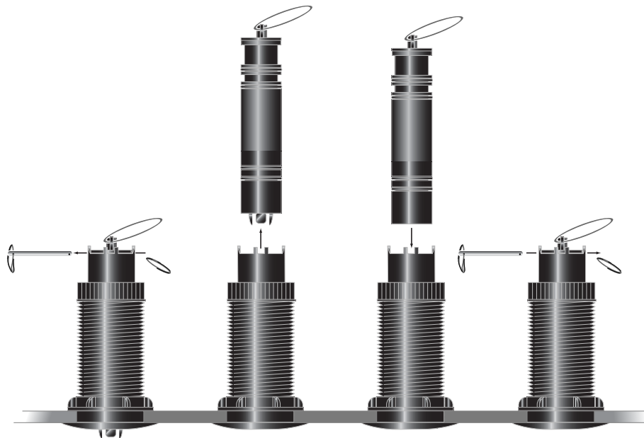
Fig 4.14 - Withdrawing the Paddlewheel Assembly
