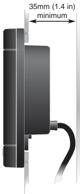
Fig 4.2 - Clearance Required Behind Bulkhead
